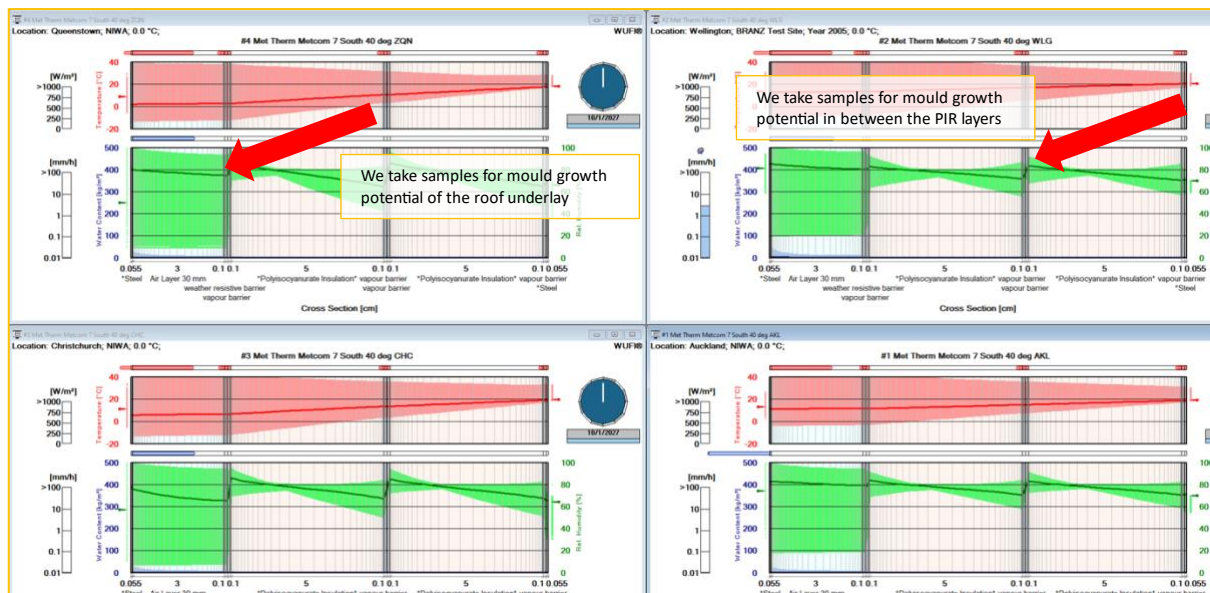
Roof section in WUFI, 40 degrees roof pitch orientated to South across Auckland, Wellington, Christchurch and Wellington
