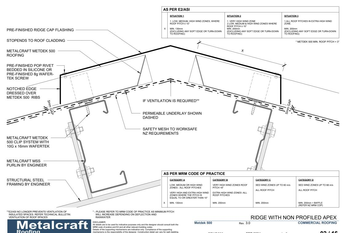
The underlay is detailed as a single line for simplicity and is indicative only. Building paper type
