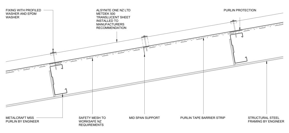
FIXING AND MID SPAN SUPPORT AS PER ALSYNITE ONE NZ LTD LITERATURE WWW.ALSYNITE.CO.NZ
