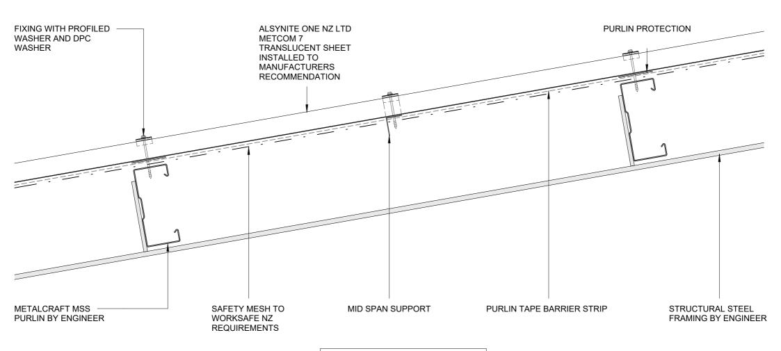
FIXING AND MID SPAN SUPPORT AS PER ALSYNITE ONE NZ LTD LITERATURE WWW.ALSYNITE.CO.NZ
