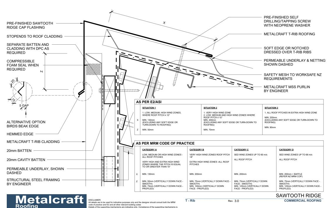
the responsibility of the designer. Construction detail can vary for wall cladding. The underlay is detailed
