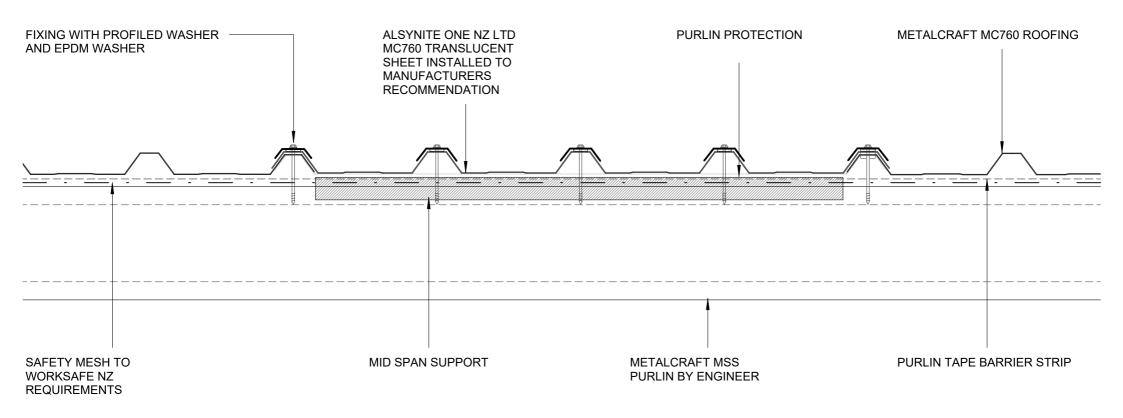
FIXING AND MID SPAN SUPPORT AS PER ALSYNITE ONE NZ LTD LITERATURE WWW.ALSYNITE.CO.NZ
