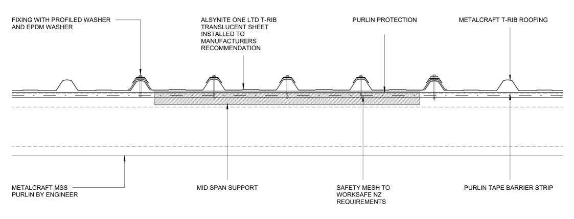
FIXING AND MID SPAN SUPPORT AS PER ALSYNITE ONE LTD LITERATURE WWW.ALSYNITE.CO.NZ
